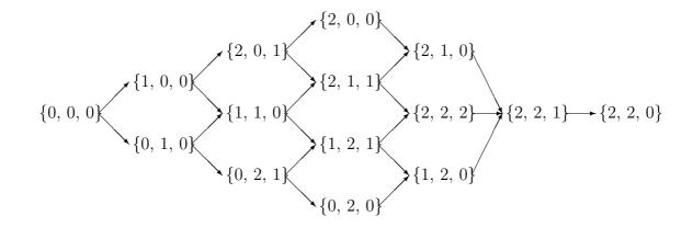
Figure 5: The state space, S, and the acceptable transitions
