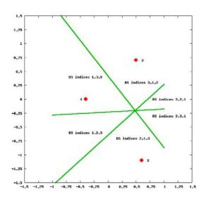
Figure 7: Using three BSs with the strongest signal
