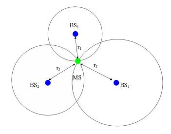
Figure 8: Triangulating the position of the handset
