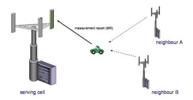
Figure 1: A measurement report being sent to the serving base station
