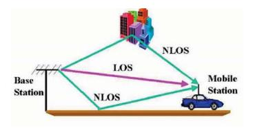
**Figure 2:** A signal from a base station can travel either by a line-of-sight path (LOS) or by non-line-of-sight (NLOS) paths
