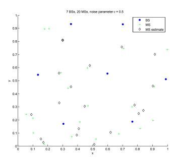
**Figure 10:** Triangulating positions of handsets with unknown transmission heights
