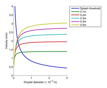
Figure 1: A regime diagram showing the experimentally determined condition for the onset of splashing for a droplet of Sarin, with splashing predicted for impacts above the solid blue line. Also shown are the impact speeds for droplets released from rest from 0.1, 0.2, 0.3, 0.4 and 0.5 m above the substrate.
