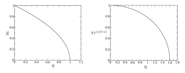
Figure 8: Shapes of self-similar solutions for the case n = 2. Short-time solution when droplet is not fully absorbed (left) and long-time solution after droplet has been absorbed (right).
