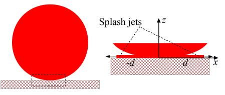
**Figure 4:** An idealized liquid droplet impacting on a solid surface, showing the formation of splash jets running over the solid surface.
