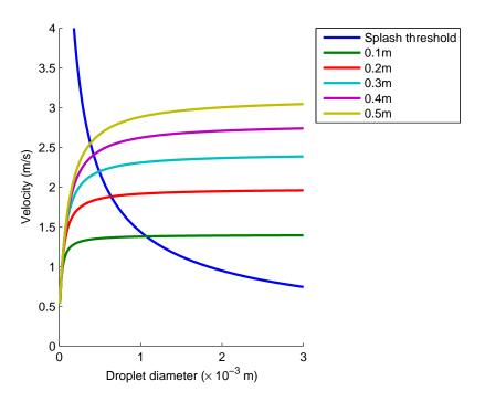
Figure 2: As figure 1, but showing the splashing threshold and impact speeds for droplets of sulphur mustard.
