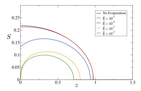
Figure 12: Numerical solutions of Richards' equation for n = 2 after the drop has been fully absorbed, showing the effects of evaporation from the surface z = 0 for different values of the scaled evaporation rate  $\hat{E} = E/D_0$  after time  $t = 5\phi/D_0$ .
