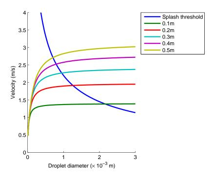
Figure 3: As figure 1, but showing the splashing threshold and impact speeds for droplets of VX.
