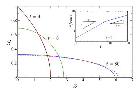
Figure 9: Numerical solution of Richards' equation with n = 2 (solid lines). The drop is fully absorbed into the porous medium at t = 5. Short and long time similarity solutions are also shown (dashed lines) and are in good agreement with the full numerical solution. The spreading of the front is observed to slow from  $t^{1/2}$  to  $t^{1/4}$  once the droplet is fully absorbed (inset).
