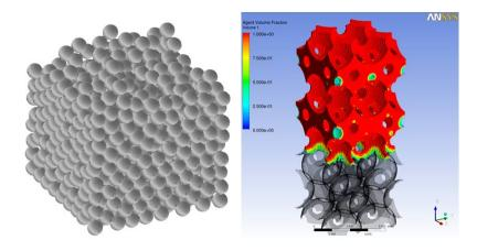
Figure 13: Existing DSTL simulations of liquid infiltration into a porous medium.
