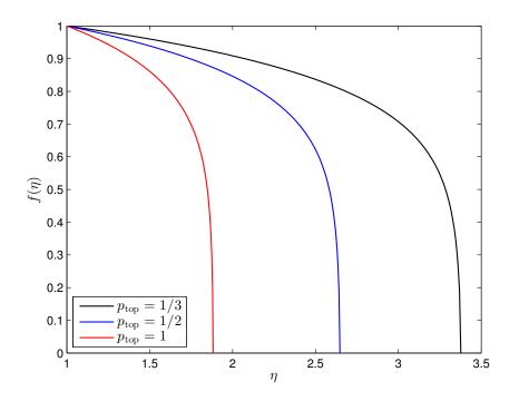
Figure 11: Saturation profiles for different values of  $p_{top}$  and for the diffusivity given in (43). See text for details of the calculation.
